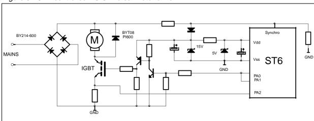
Figure 6. IGBT controlled DC Universal motor drive.
