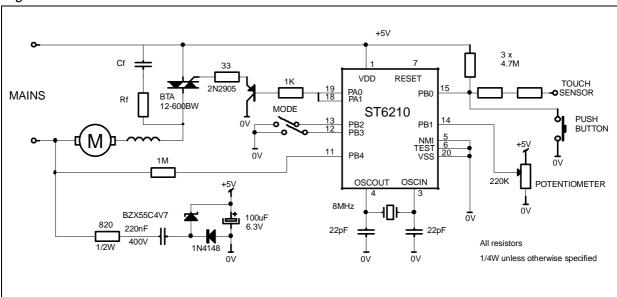
Figure 4. TRIAC controlled AC mode Universal motor drive
