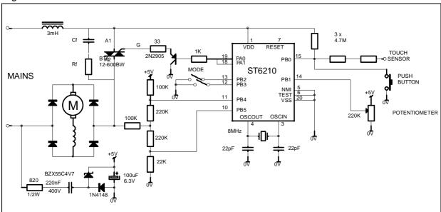
Figure 5. TRIAC controlled DC mode Universal motor drive
