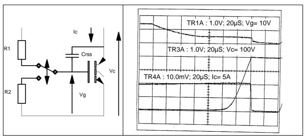
Figure 7b. Control of IGBT Switching behaviour
