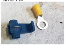
Used 18-16 GA Moisture Resistant Tap Connector Remove Spade Used small file to open center
